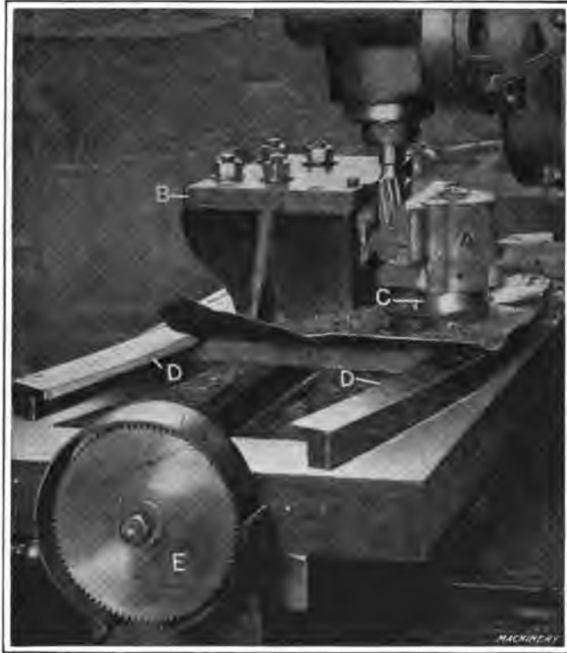
Fig. 17. Fixture for Milling Curved Slot in Sight-bar Bracket
